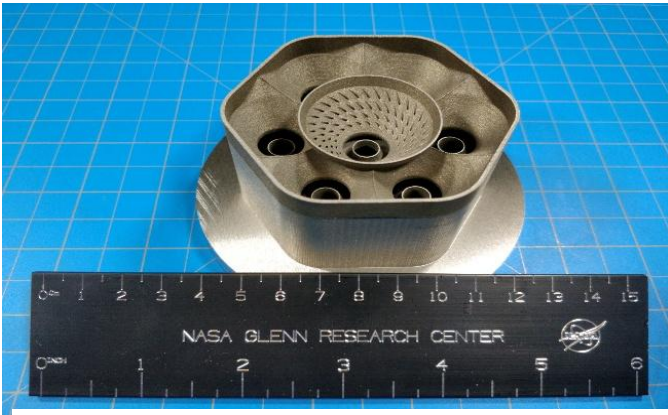
NASA photo of 3D-made GRX-810 alloy part.
